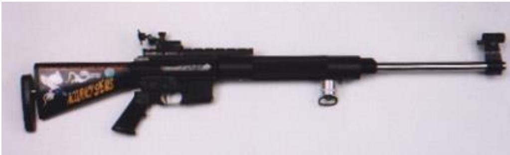
The AR15 is a match rifle built on an AR15 platform. It has the aperture sights, free float tube with handstop and an adjustable buttplate. These can be made in various configurations, this is just a modest example to show what can be done. It is probably chambered in 223 Remington. Rifles similar to this can be built on an AR10 platform as well and chambered in calibers suitable for that action, i.e. 308, 243, 264 Rem., 708, 22-250, etc.
