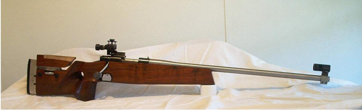
Bill Rodolph's rifle is built on a short action, Winchester Model 70. It has an Anschutz trigger, Krieger barrel and at present is chambered in 22BR. It is pillar bedded in a copy of an Anschutz 1813 Supermatch stock. The cheekpiece and butt are adjustable and the hardware was made by Bill and the rifle was completely gunsmithed by Bill Rodolph. It is reloaded in rapid fire matches from the top with a stripper clip.
